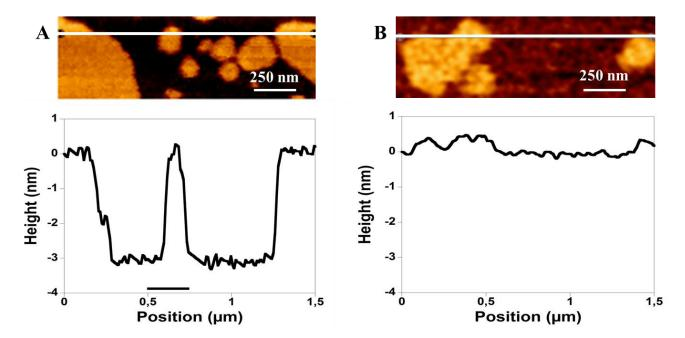
**Figure S2:** AFM images and cross-section profiles of *E.coli* lipid extract vesicles incubated 30 minutes on mica substrate, by tapping mode (A) and contact mode (B). The images size is  $0.5 \times 1.5 \mu m$ . Height value for *E.coli* lipid patches by tapping mode is 3-4 nm, and height value by contact mode is about 0.5 nm.
